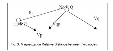
Node P velocity is Vp and Node Q velocity is Vq initial distance between P and Q is R after  $\Delta t$  sec the distance between P and Q we call as Relative distance between P and Q.
